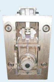
mechanism disregard traditional male-female structure and instead employ a face-contact design to maximize the area between nozzle and sliding plates. Face pressure is stabilized increasing safety and ease of application and disassembly.
