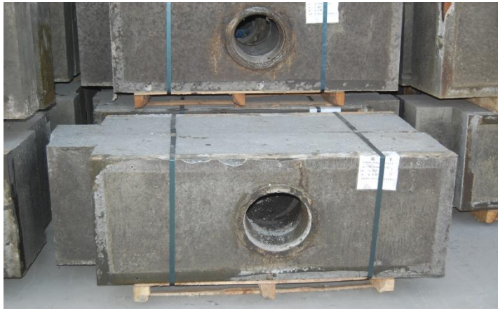
Precast blocks / 预制炉面块
